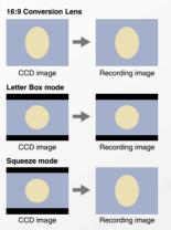
Activating the Aspect Ratio function on the LCD allows for a letterbox display for easier framing when shooting in Squeeze Mode or when using the Anamorphic lens.
